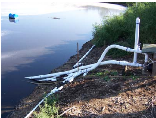
Figure 2. The aerator module in the field test
