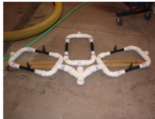
Figure 3. The configuration of the aerator module
