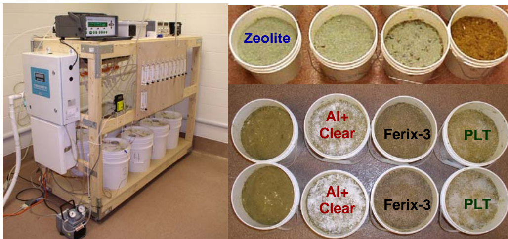
Figure 1. Emission vessels system used to evaluate efficacy of various manure treatment agents to reduce ammonia emissions from manure storage.
