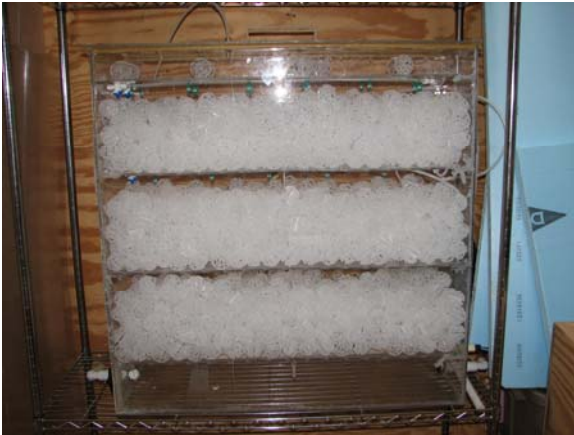
Figure 1. Bioscrubber setup (lab scale)
